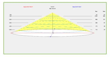
The Illuminance Cone Diagram indicates the maximum illuminance at different distances from the fixture.
